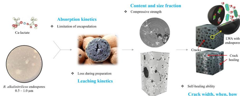
Figure 1: Strategy to design and test a microbially-engineered self-healing cement system.
