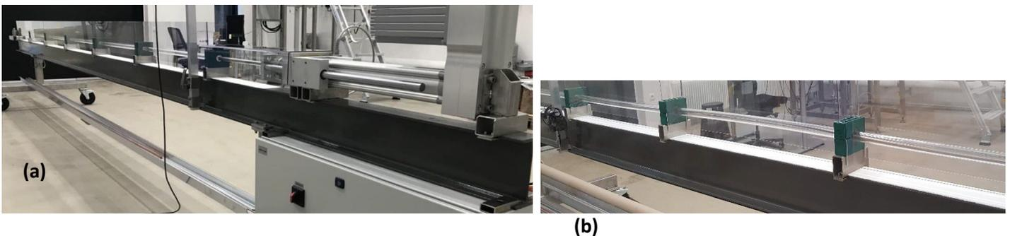
Figure 1: (a) Lab scale set-up of the CT and well casing, (b) steel CT buckling inside the PMMA casing
