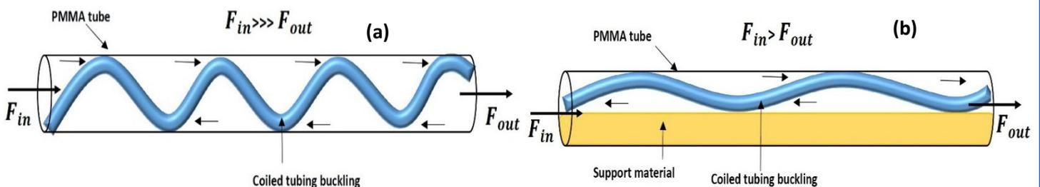
Figure 2: Schematic representation of (a) coiled tubing buckling inside PMMA tube and (b) coiled tubing buckling inside PMMA tube filled with support material.  $F_{in}$  is 'Force in' and  $F_{out}$  is 'Force out'.
