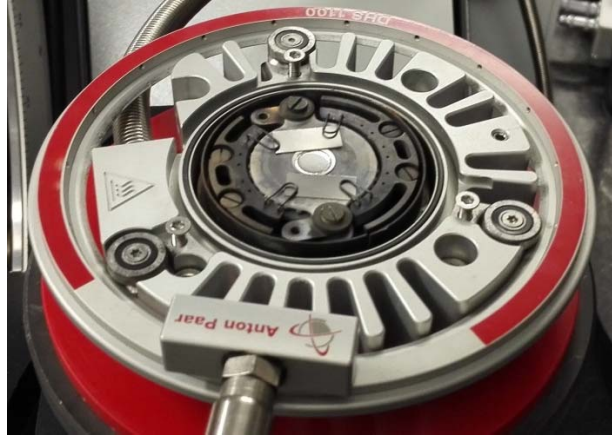
Figure 3.8: Heating stage for in-situ high temperature investigation with a loosely fixed, disc-shaped sample. Before measurements, the heating stage was enclosed by a graphite dome, evacuated and purged with Ar, and exposed to a low and continuous Ar flow during acquisition.
